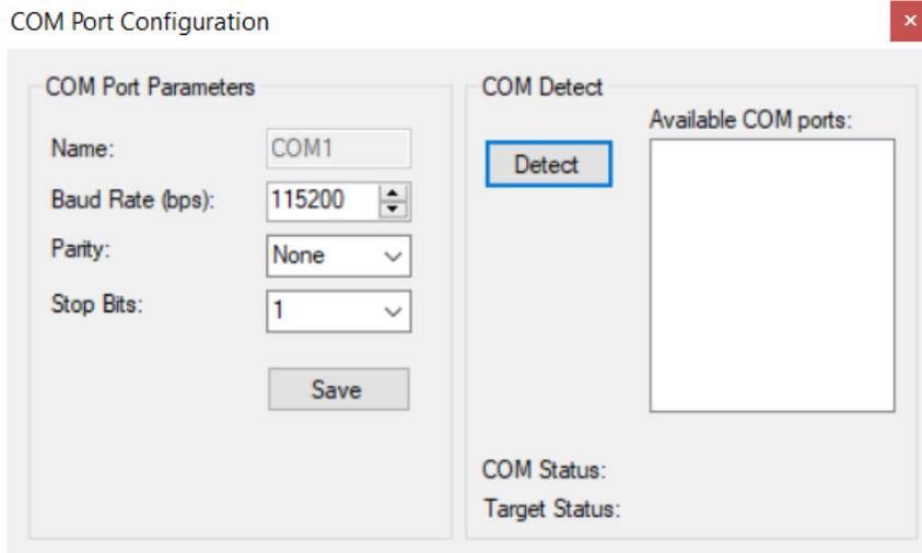
The PAC BMS FW is configured to use the default UART parameter values shown in the **COM Port Parameters** dialog box, namely 115200 bps, no Parity, and 1 Stop Bit.
