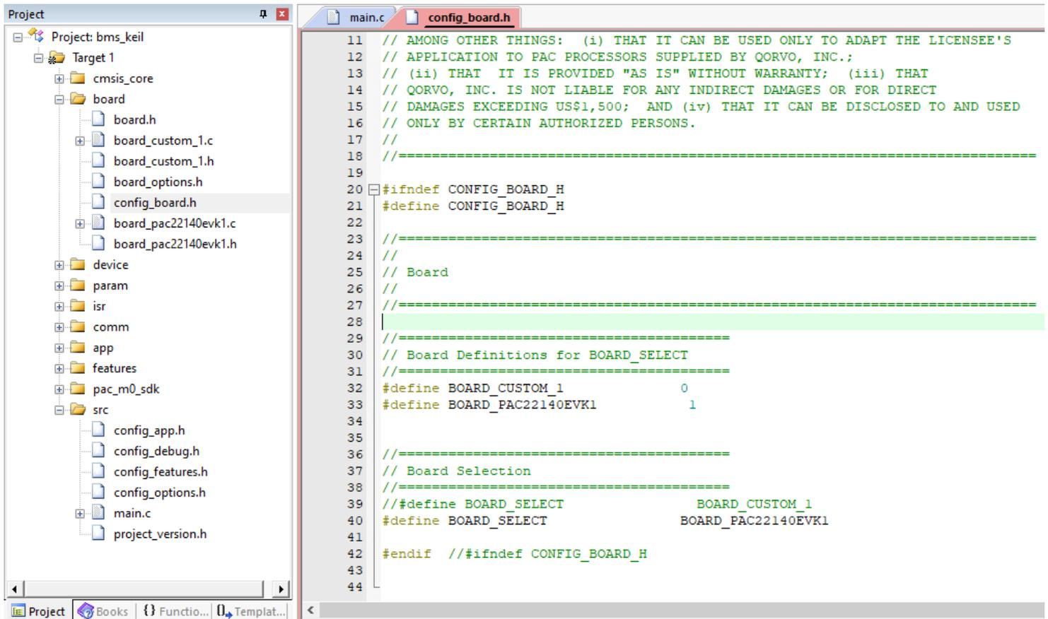
provided to configure the BMS FW. Open the config\_board.h file in board folder and navigate to the “Board Selection” portion of the code. Uncomment the BOARD\_SELECT for the desired PAC EVK and comment out all other BOARD\_SELECT lines. In the example below, the PAC22140EVK1 has been chosen.
