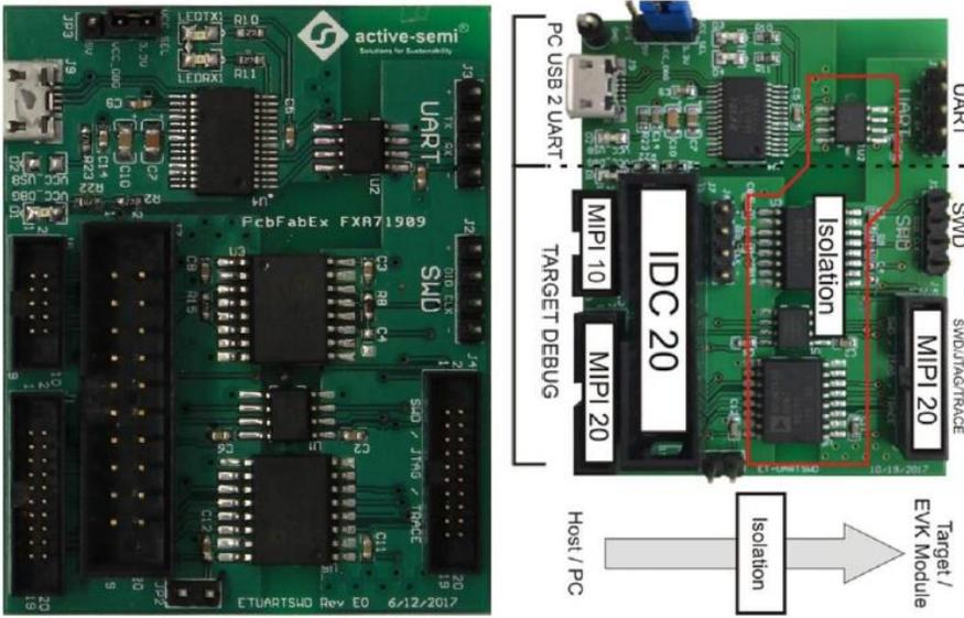
To connect the UART, use a 4-wire cable to connect the PAC EVK 4-pin UART header labelled [ + TX RX - ] to the ET-UARTSWD 4-pin UART header labelled [ + TX RX - ]. The image on the right shows the connections for the PAC22140 EVK.
