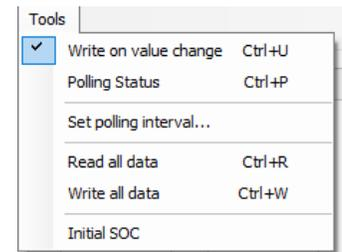
To initialize SOC starting point which is match to SOC profile curve, click **Initial SOC** in **Tools** before enable FETs control.
