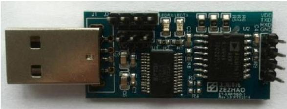
To connect the UART, use a 4-wire cable to connect the PAC EVK 4-pin UART header labelled [ + TX RX - ] to the ET-UARTISO-1 4-pin UART header labelled [ V T R G ]. Note that V T R G stands for Vcc, Tx, Rx, and Gnd respectively. Then, connect the USB port to a PC.
