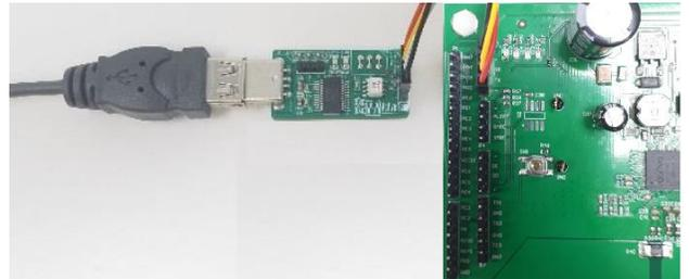
LEDTX and LEDRX LEDs will turn on and off based on UART TX and RX activity respectfully.
