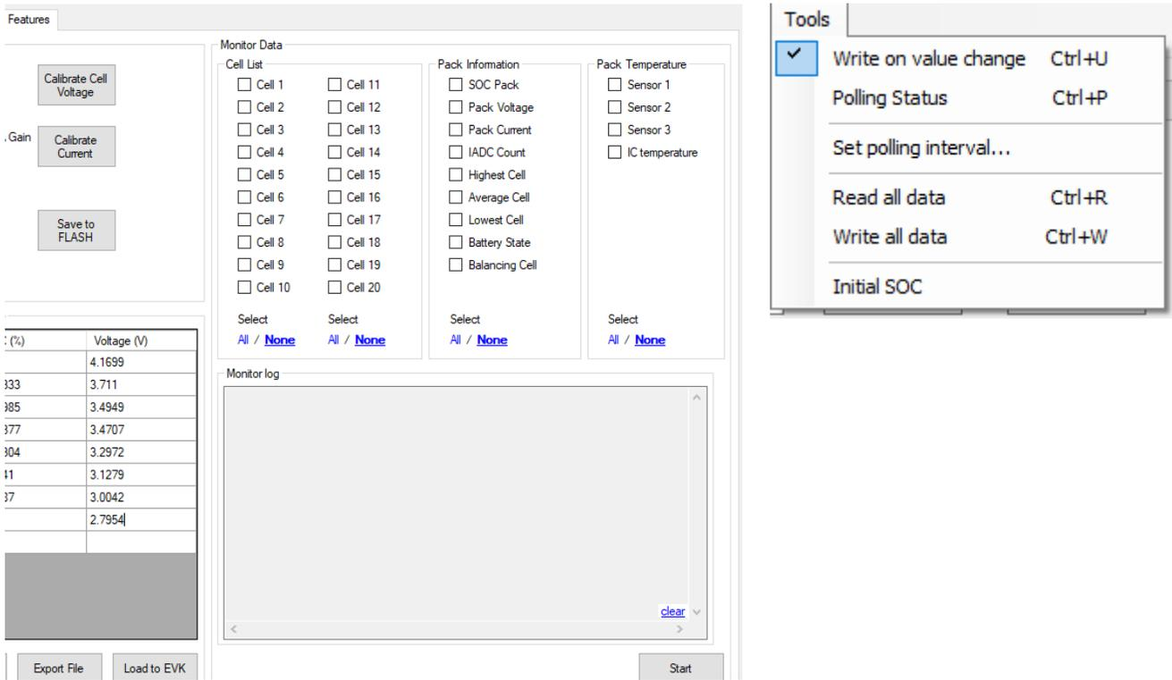
Click **Start** button to start logging file after all expected parameters are selected, the button **Start** will change to **Stop** button. The log file is saved in folder which contains execute BMS\_GUI.exe. To stop the logging process, click **Stop** button. The image below is an example output format of data log file.
