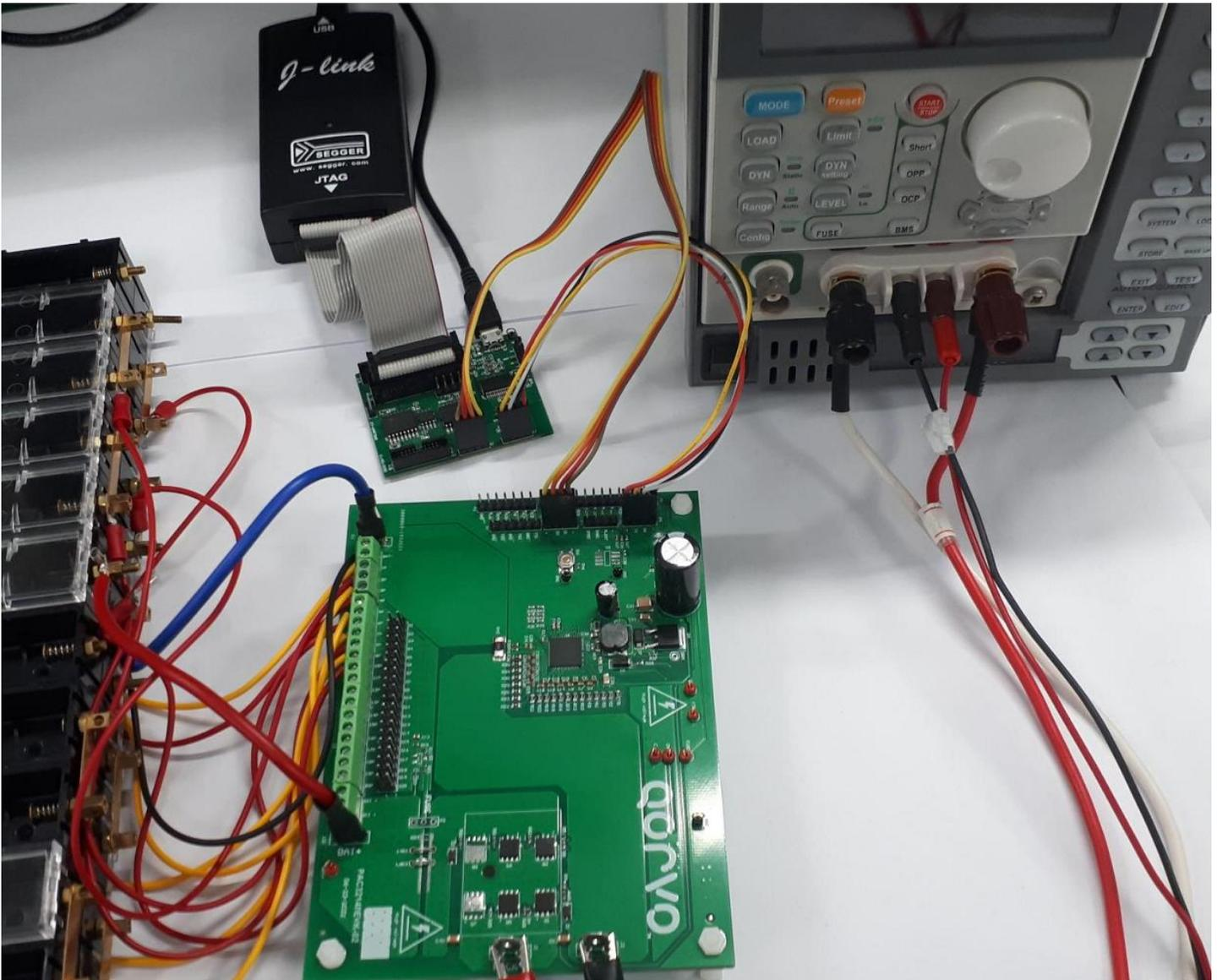
VBx Connection note: The VBx cells sense may be wrapped and plug to J7 and J8 header connectors instead of using screw connectors.
