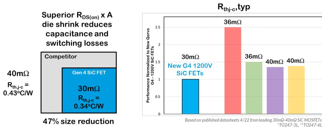
Figure 2 Comparative junction-to-case thermal performance of new 1200V Gen 4 SiC FETs with competing 1200V FET by employing advanced Ag-sintering technology
