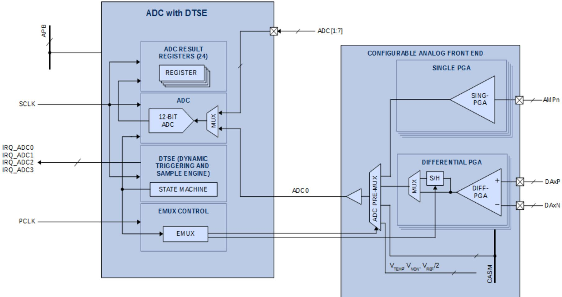
EMUX Settling issues only come into play when converting ADC0
