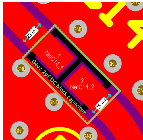
Figure 11. DC block capacitor matching to RF Trace
