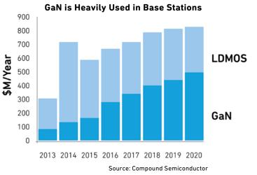
With more than one GaN process to choose from, a designer can optimally match a GaN technology to an application. The graph below examines Qorvo's capabilities in this realm.
