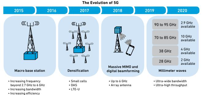
Figure 1. A number of technologies will be required to optimize performance in 5G wireless networks, including distributed antenna systems (DAS), millimeter-wave technology, and small cell base stations.
