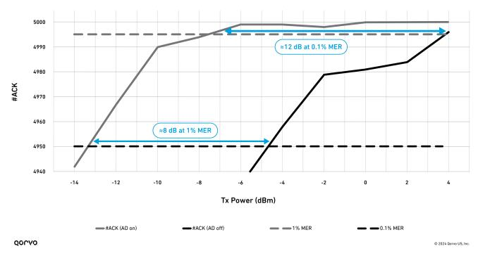
Figure 9: Range test with and without Rx antenna diversity enabled for ACK reception.
