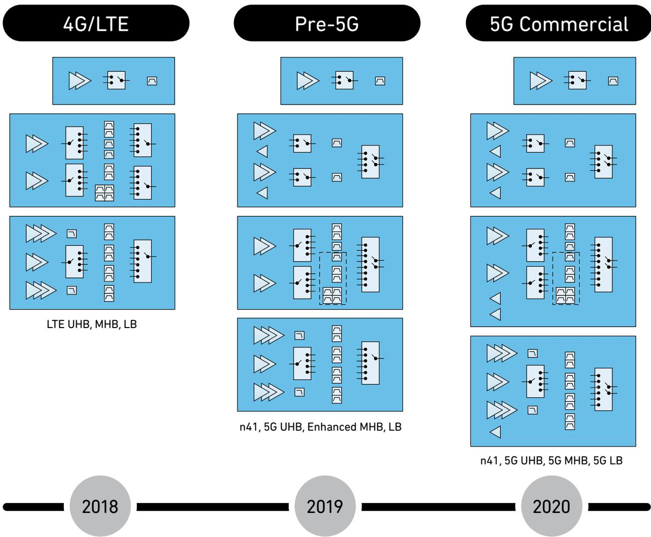
Advanced LTE and pre-5G front-end architectures add content and increase antenna complexity, compounding losses in transmit and receive paths. New modulation schemes require more linear power than ever before. RF Fusion delivers industry-leading performance in fully proven integrated systems to enable and optimize the next wave of high-performance smartphones and connected devices.
